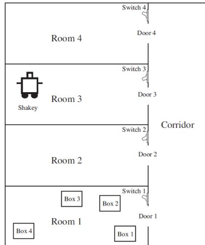
The actions in Shakey's world include moving from place to place, pushing movable objects (such as boxes), climbing onto and down from rigid objects (such as boxes), and turning light switches on and off. The robot itself could not climb on a box or toggle a switch, but the planner was capable of finding and printing out plans that were beyond the robot's abilities. Shakey's six actions are the following:
